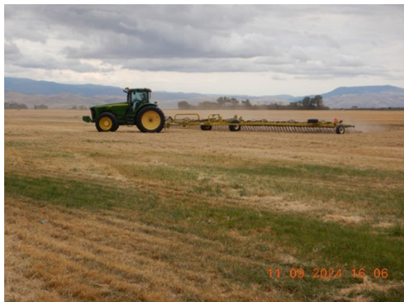
Figure 3. Degelman Strawmaster 70-foot wide heavy harrow with 26" spring-mounted tines.
